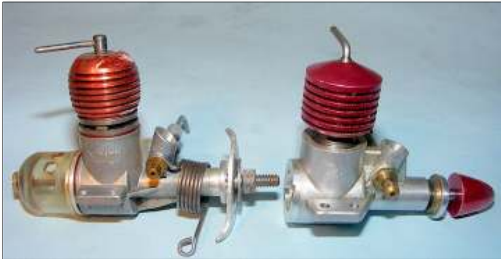
Fig 10. The PAW 55 De Luxe (R) beside a standard DC Quickstart Dart-even with the integral tank, quickstart spring and tank- the Dart is still lighter at 44g compared to the PAW's 50-powerwise though the PAW is much more powerful-by some 40%...mounting hole and bearer spacing is identical for both.
