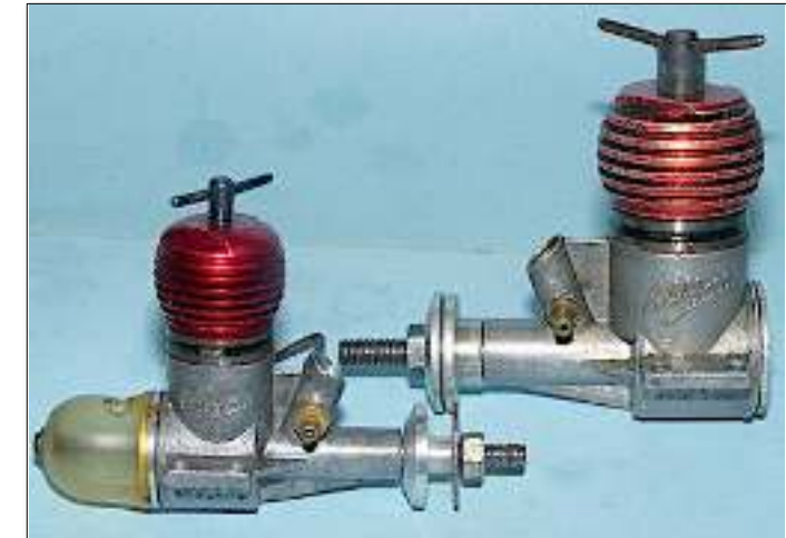
Fig 5. The Mk2 versions of the Allbon Dart and Javelin-now made by DC Ltd
