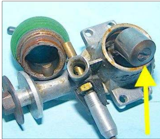
Fig 3. Dart Mk1 series 1 showing screw retention of captive gudgeon.
